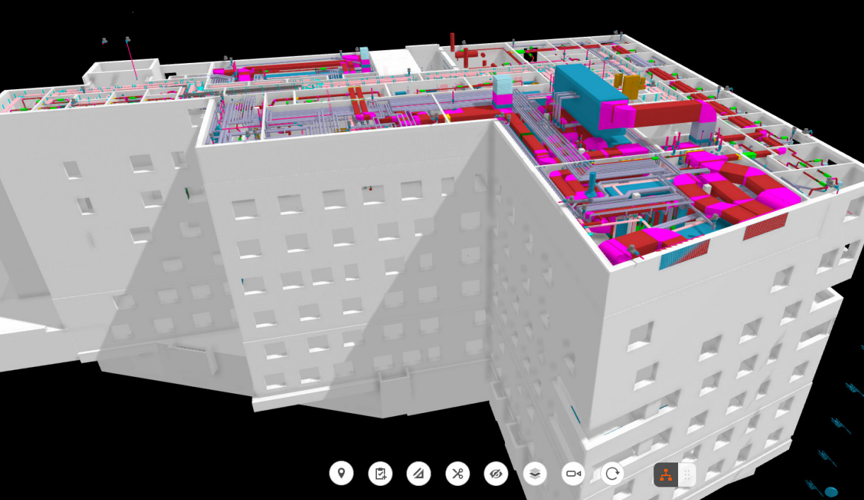
Project system in Bimplus for the connection of external specialist planners. © Schmidt Plöcker
